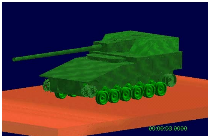
Figure 6: 18-Ton Tracked Vehicle with 120-mm Cannon
